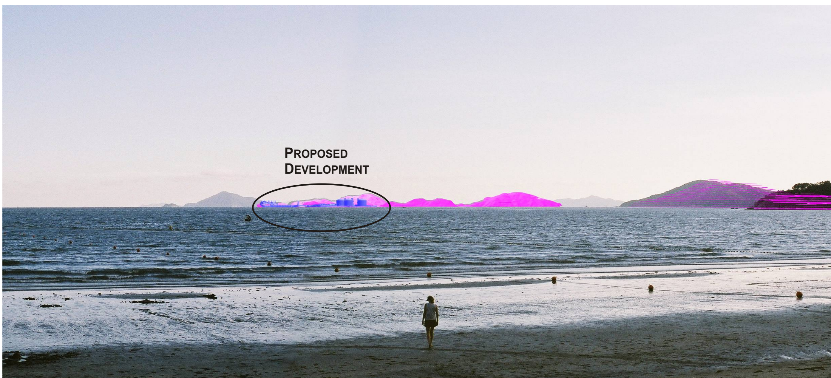
WIREFRAME OF THE PROPOSED DEVELOPMENT AND THE DIGITAL TERRAIN MODEL COMPOSITED ONTO THE PHOTOGRAPHS.
