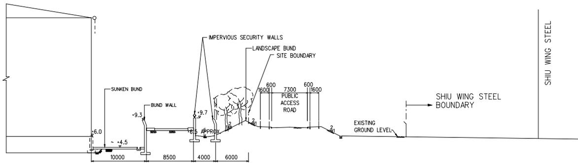
Beyond the second reinforced concrete security wall, there is an additional landscape bund which will provide additional containment for any liquids escaping over the primary bund wall and the two security walls. This is a simple earth mound as shown in the diagram, rather than a reinforced concrete structure.
