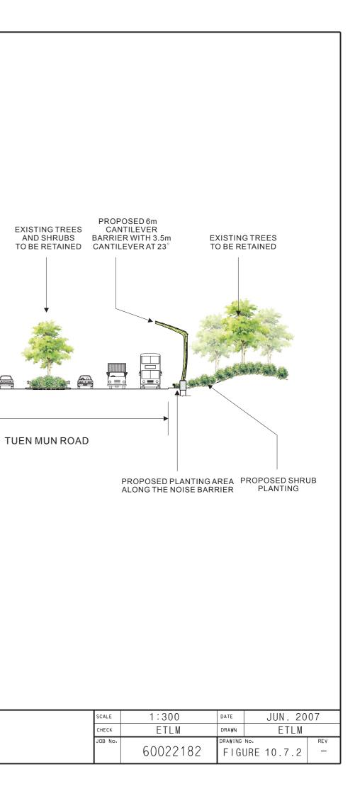
PROPOSED 6m CANTILEVER BARRIER WITH 2.5m
