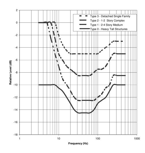
FIGURE 1 BUILDING COUPLING FACTOR - TYPE 0 TO TYPE 3 STRUCTURES
