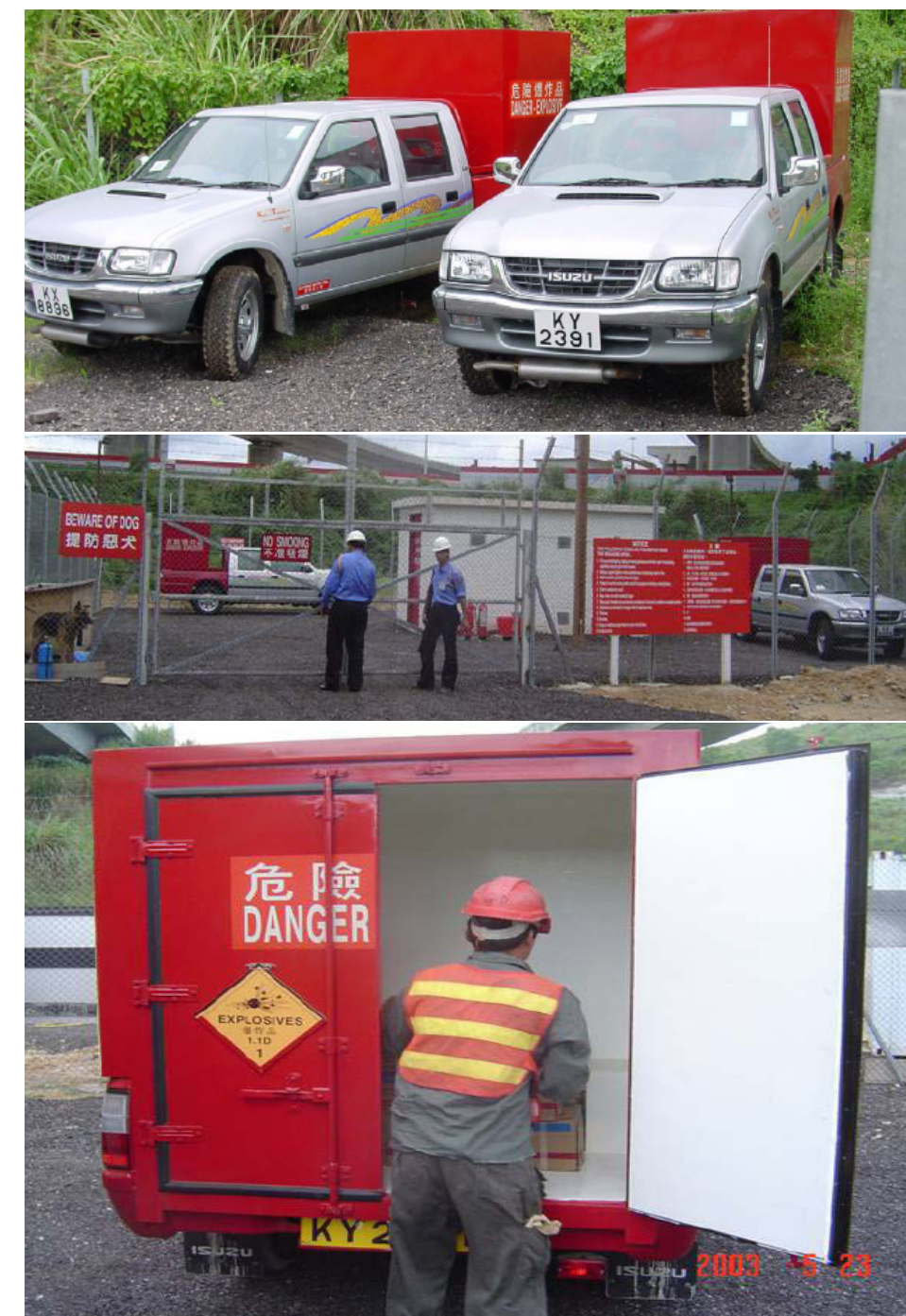
Figure 2.2 Typical Contractor’s Explosives truck and Magazine
