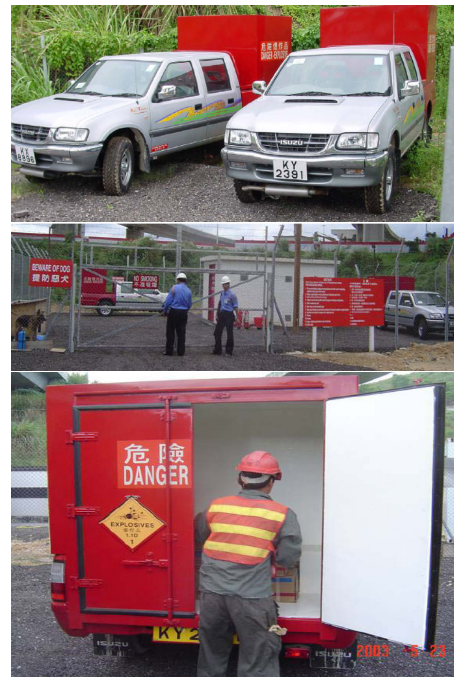
Figure 2.2 Typical Contractor’s Explosives truck and Magazine
