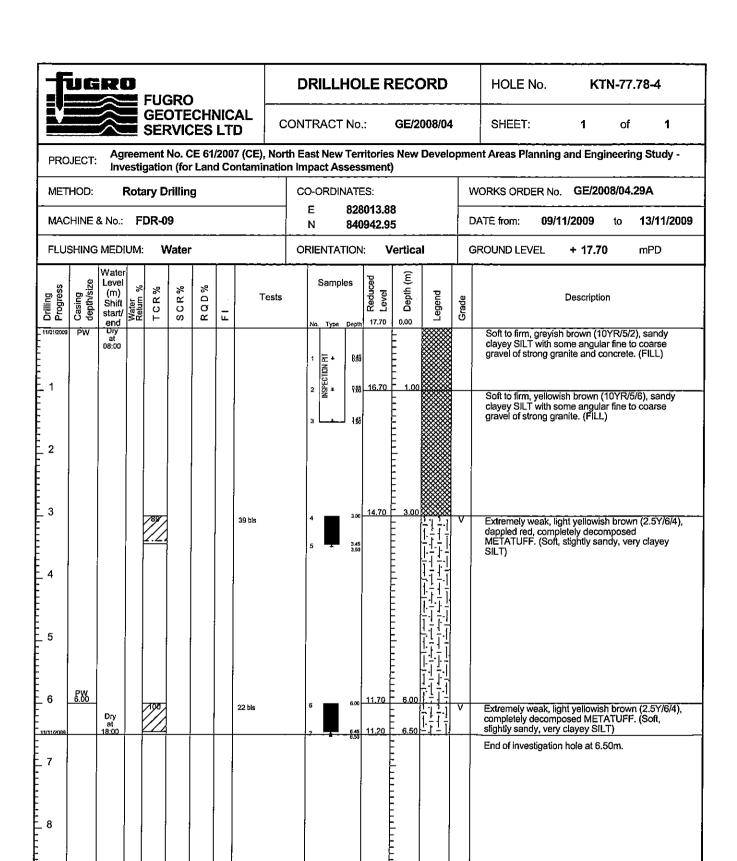
Small Disturbed Sample Piston sample U76 Undisturbed Sample U100 Undisturbed Sample Mazier Sample
