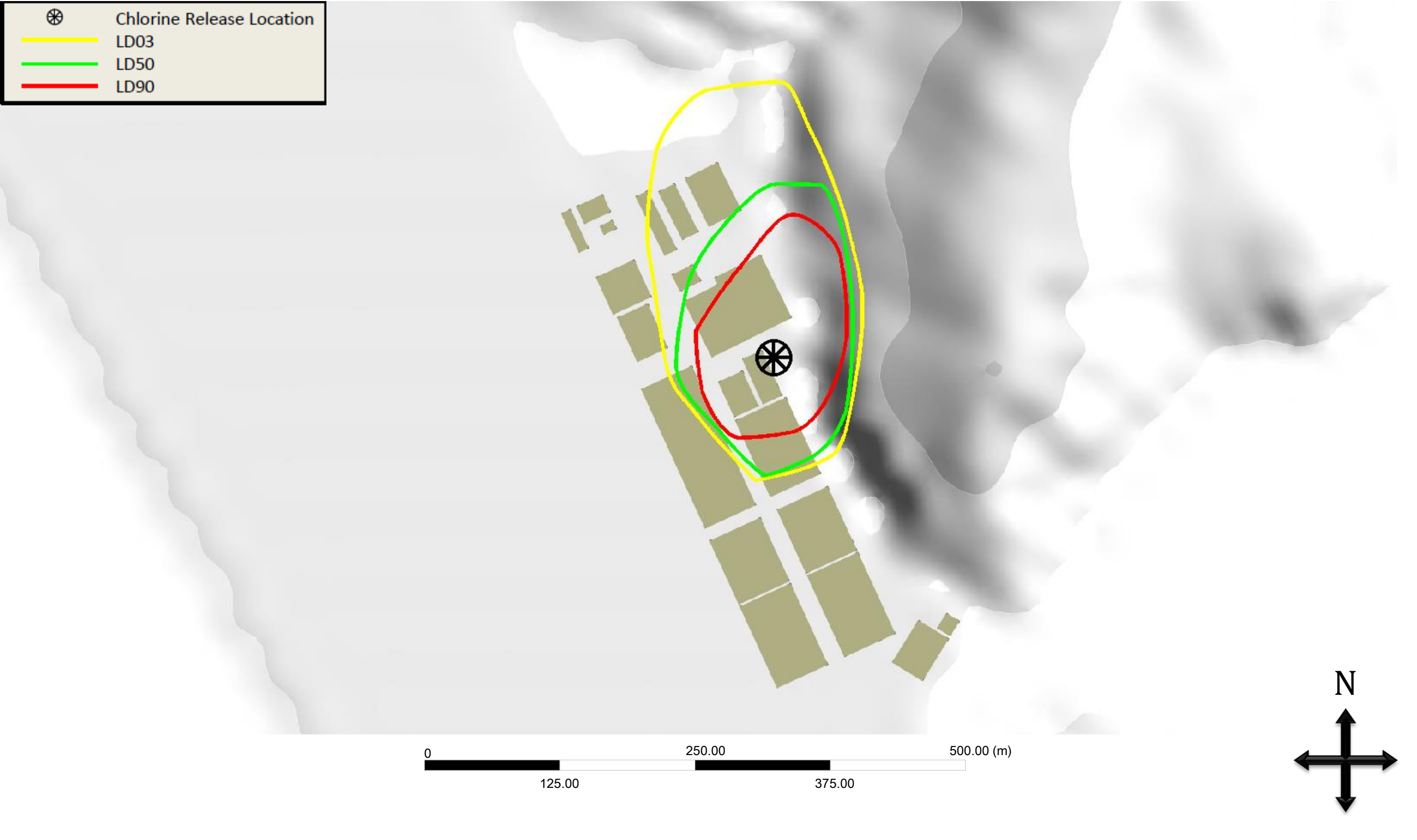
Figure 23 CFD Modelling Results for the Proposed Desalination Plant at Tseung Kwan O – Lethal Dose Contours LD03, LD50 and LD90
