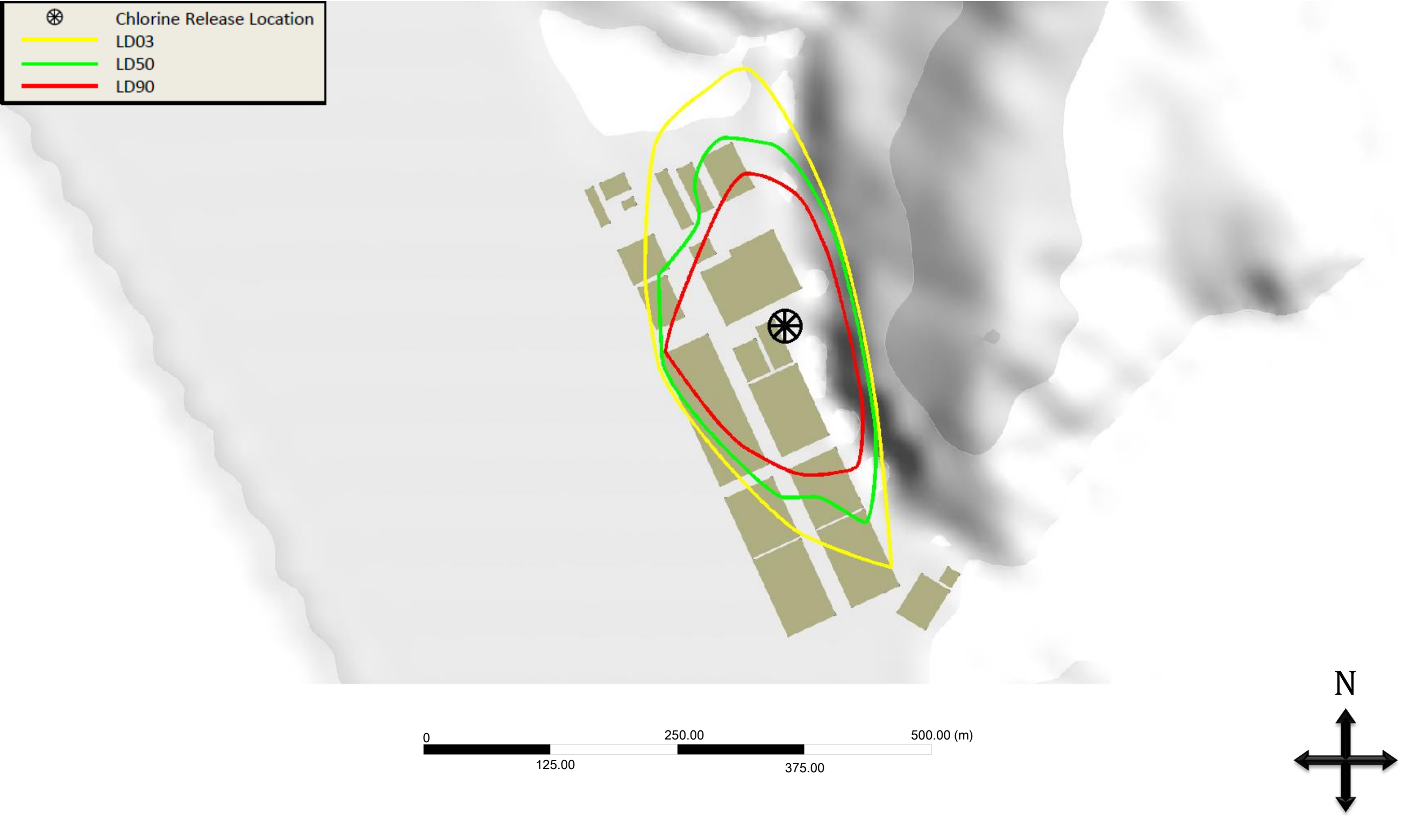
Figure 18 CFD Modelling Results for the Proposed Desalination Plant at Tseung Kwan O – Lethal Dose Contours LD03, LD50 and LD90
