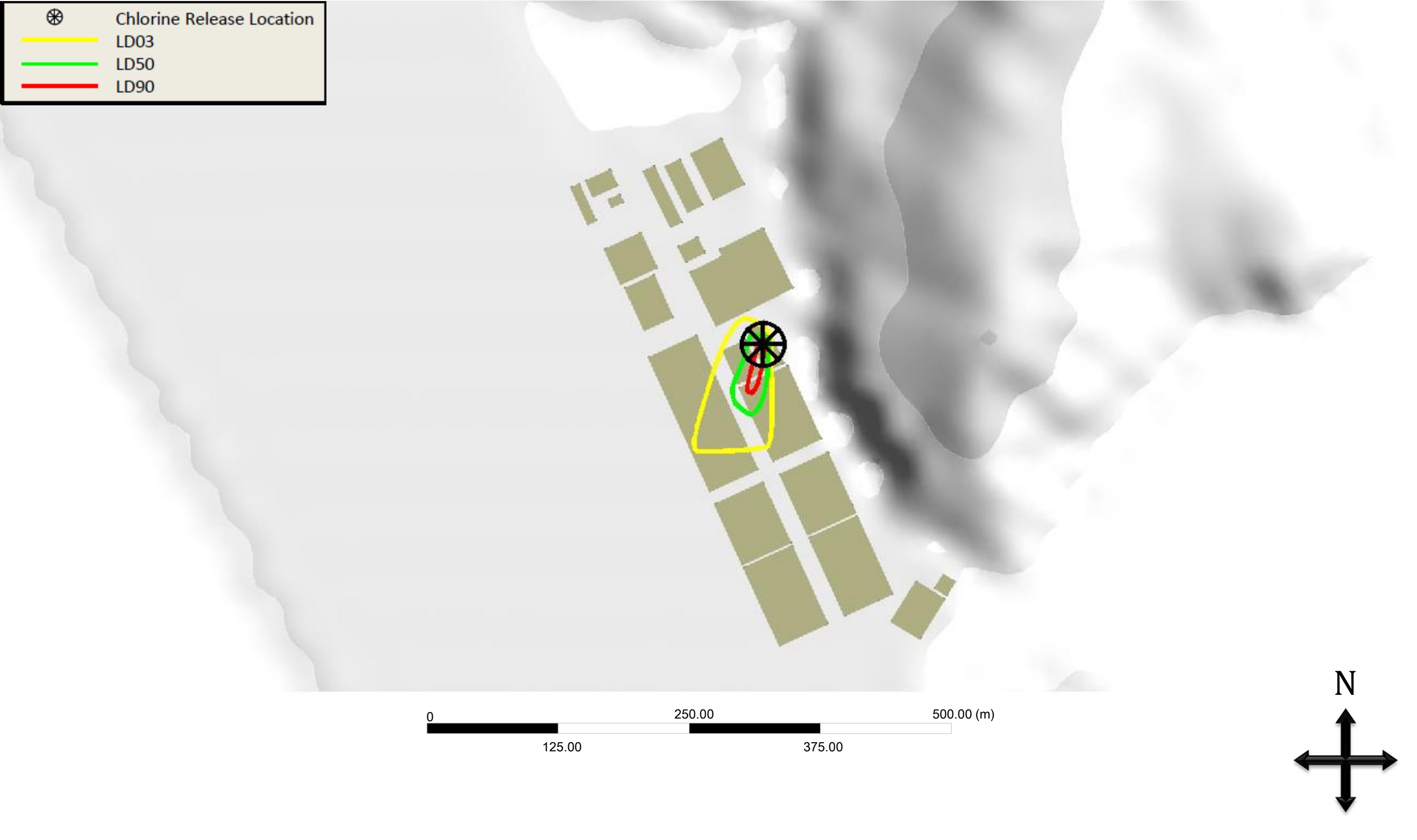
Figure 26 CFD Modelling Results for the Proposed Desalination Plant at Tseung Kwan O – Lethal Dose Contours LD03, LD50 and LD90
