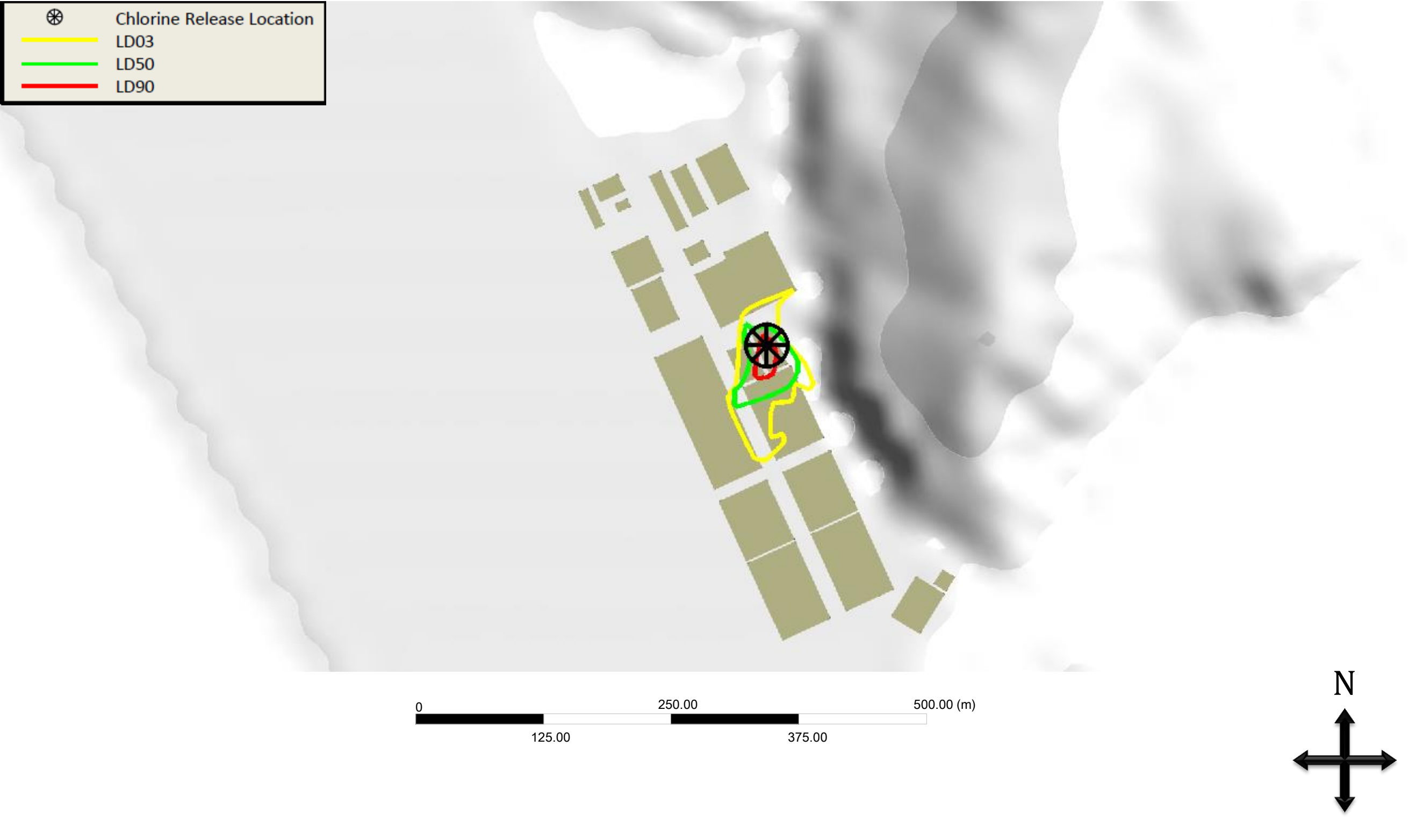
Figure 25 CFD Modelling Results for the Proposed Desalination Plant at Tseung Kwan O – Lethal Dose Contours LD03, LD50 and LD90
