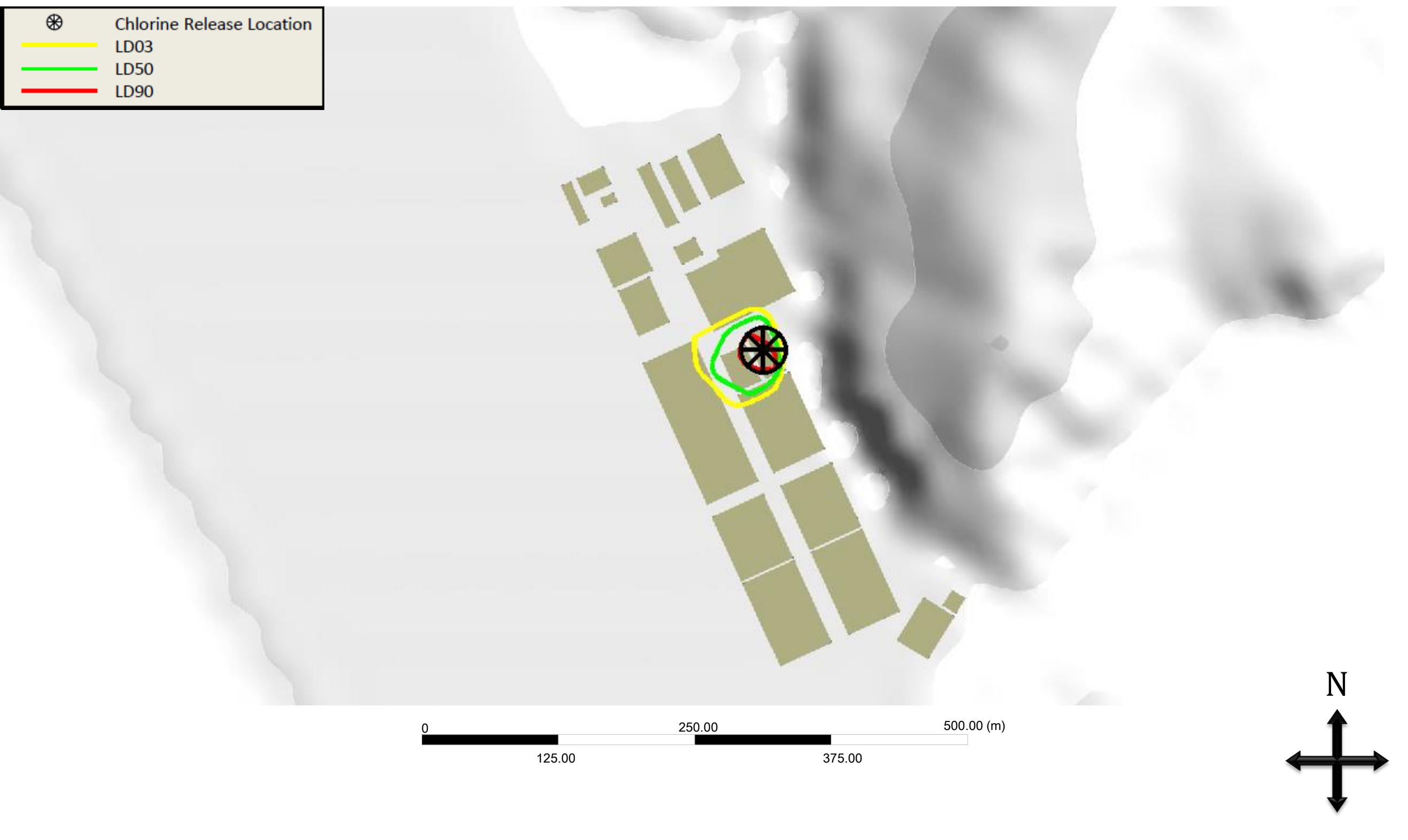
Figure 30 CFD Modelling Results for the Proposed Desalination Plant at Tseung Kwan O – Lethal Dose Contours LD03, LD50 and LD90
