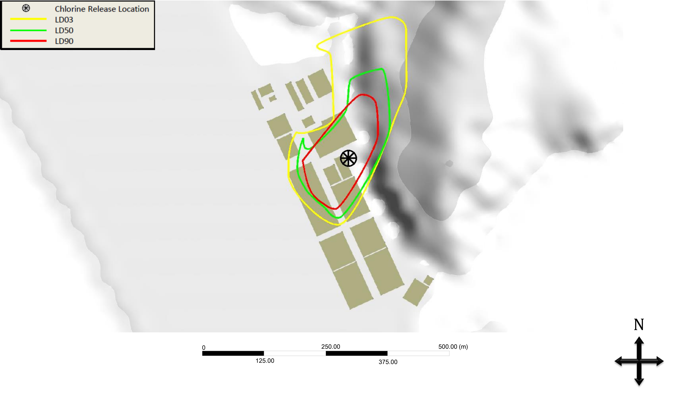
Figure 22 CFD Modelling Results for the Proposed Desalination Plant at Tseung Kwan O – Lethal Dose Contours LD03, LD50 and LD90
