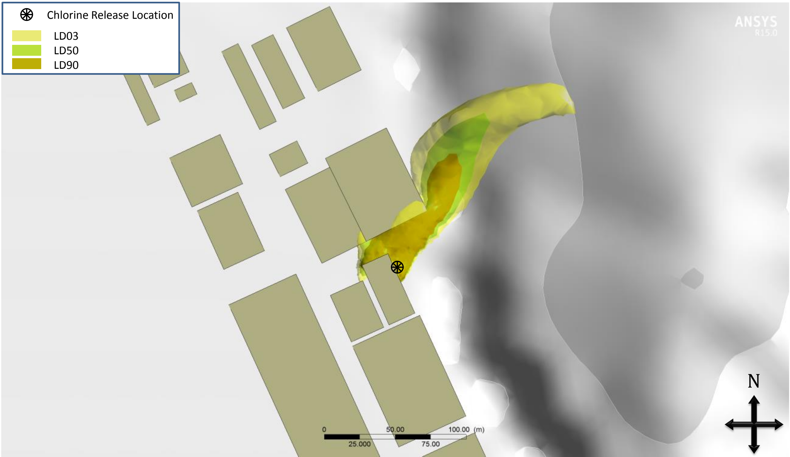
Figure 9 CFD Modelling Results for the Proposed Desalination Plant at Tseung Kwan O – Lethal Dose Contours LD03, LD50 and LD90
