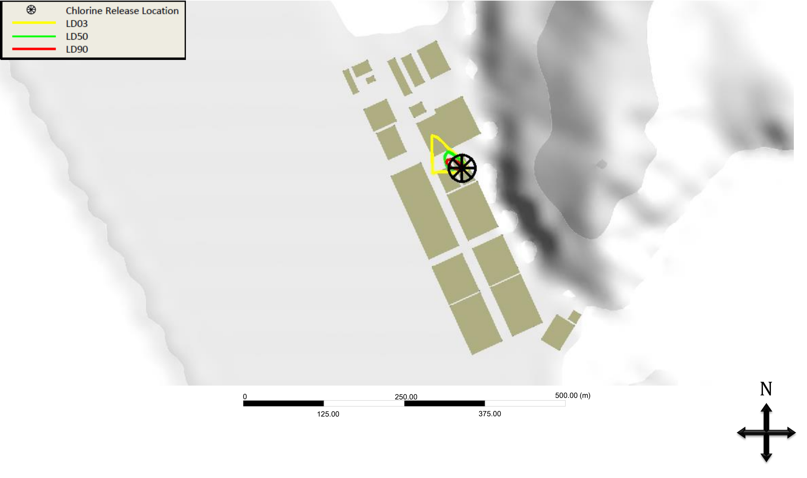
Figure 34 CFD Modelling Results for the Proposed Desalination Plant at Tseung Kwan O – Lethal Dose Contours LD03, LD50 and LD90
