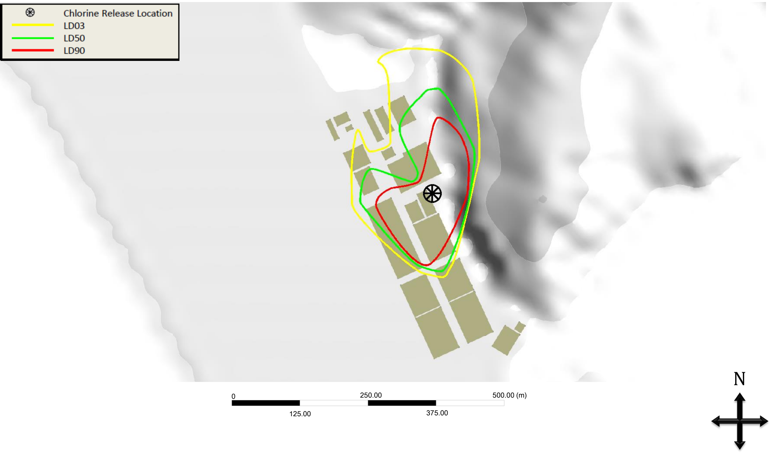
Figure 16 CFD Modelling Results for the Proposed Desalination Plant at Tseung Kwan O – Lethal Dose Contours LD03, LD50 and LD90
