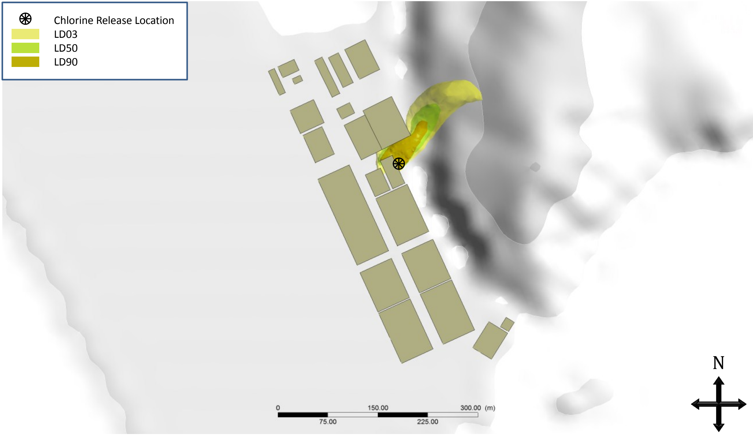
Figure 3 CFD Modelling Results for the Proposed Desalination Plant at Tseung Kwan O – Lethal Dose Contours LD03, LD50 and LD90
