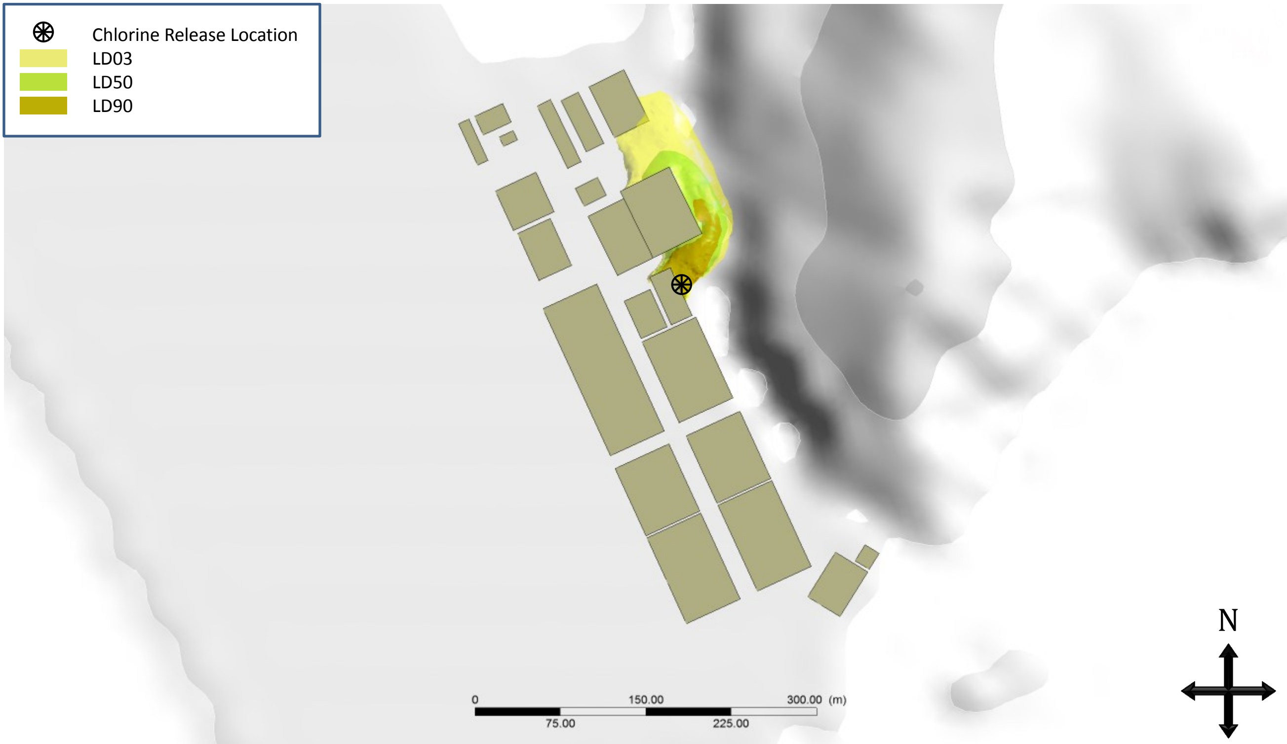
Figure 5 CFD Modelling Results for the Proposed Desalination Plant at Tseung Kwan O – Lethal Dose Contours LD03, LD50 and LD90
