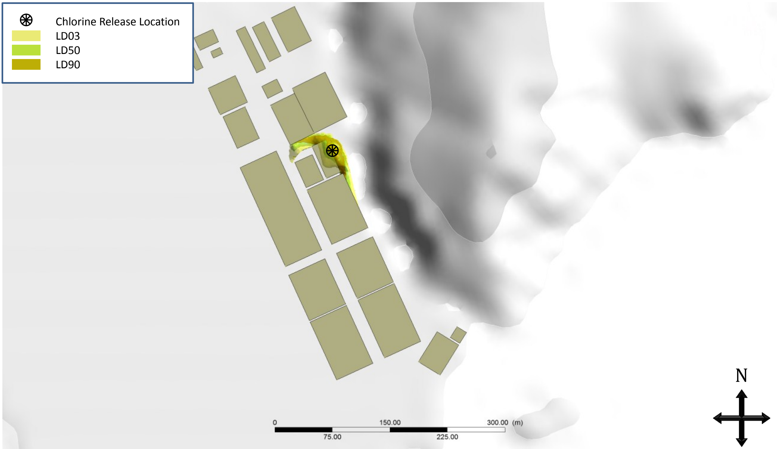
Figure 15 CFD Modelling Results for the Proposed Desalination Plant at Tseung Kwan O – Lethal Dose Contours LD03, LD50 and LD90
