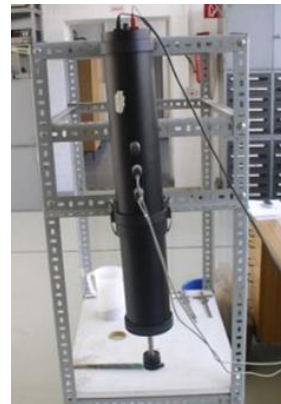
Impedance tube (Brüel & Kjær, type 4206)
