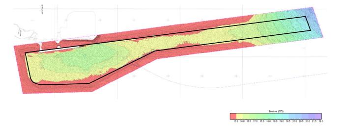
(Note: the boundary of the navigation channel is delineated by the black line. Areas shown in red have exceeded the minimum channel depth requirement as specified in the 2008 Berthing Guidelines)
