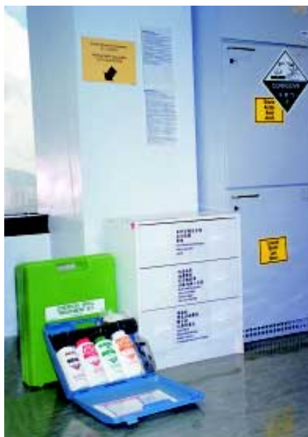
Emergency Spill Kit and guidelines for dealing with chemical spillage in the laboratory.
