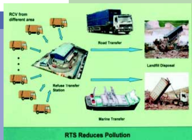
Refuse transfer stations reduce pollution from the use of a large number of small refuse collection vehicles
