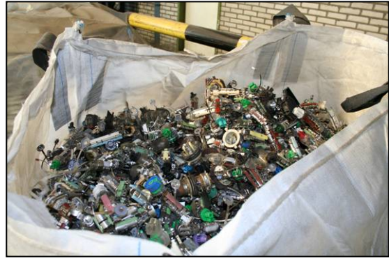
Photo no. 7: Electronic components recovered during manual disassembly of the equipment
