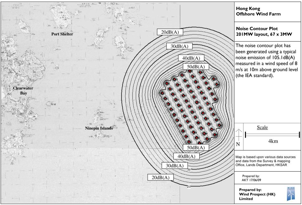
Note: The Noise Contour Plot is for the 67 turbine layout scenario. The 40 turbine layout would have a reduced noise profile and this plot is the "worst-case" scenario.
