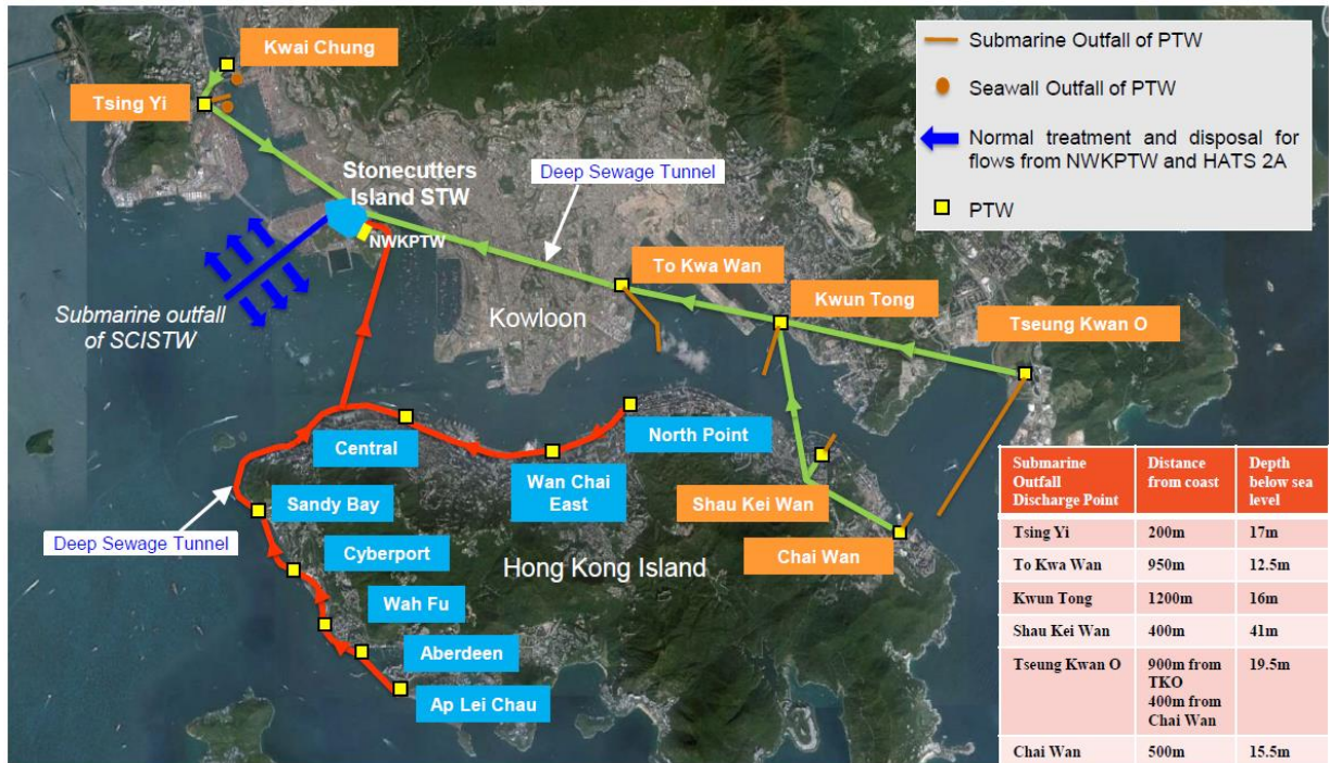
Figure A Proposed Two-week Sewage Bypass at Seven PTWs of HATS Stage 1
