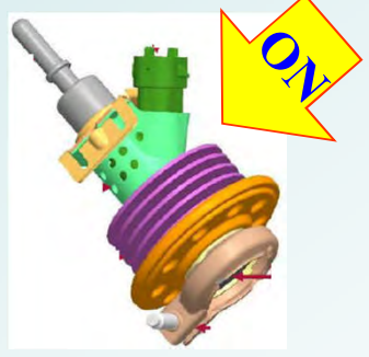
Stage 3: Dosing Module on Pump on when pressure drop
