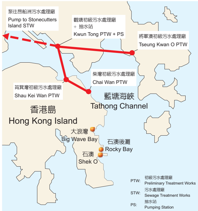
圖 4.5 改善藍塘海峽水質的淨化海港計劃工程 Figure 4.5 HATS works causing improvement of water quality at Tathong Channel
