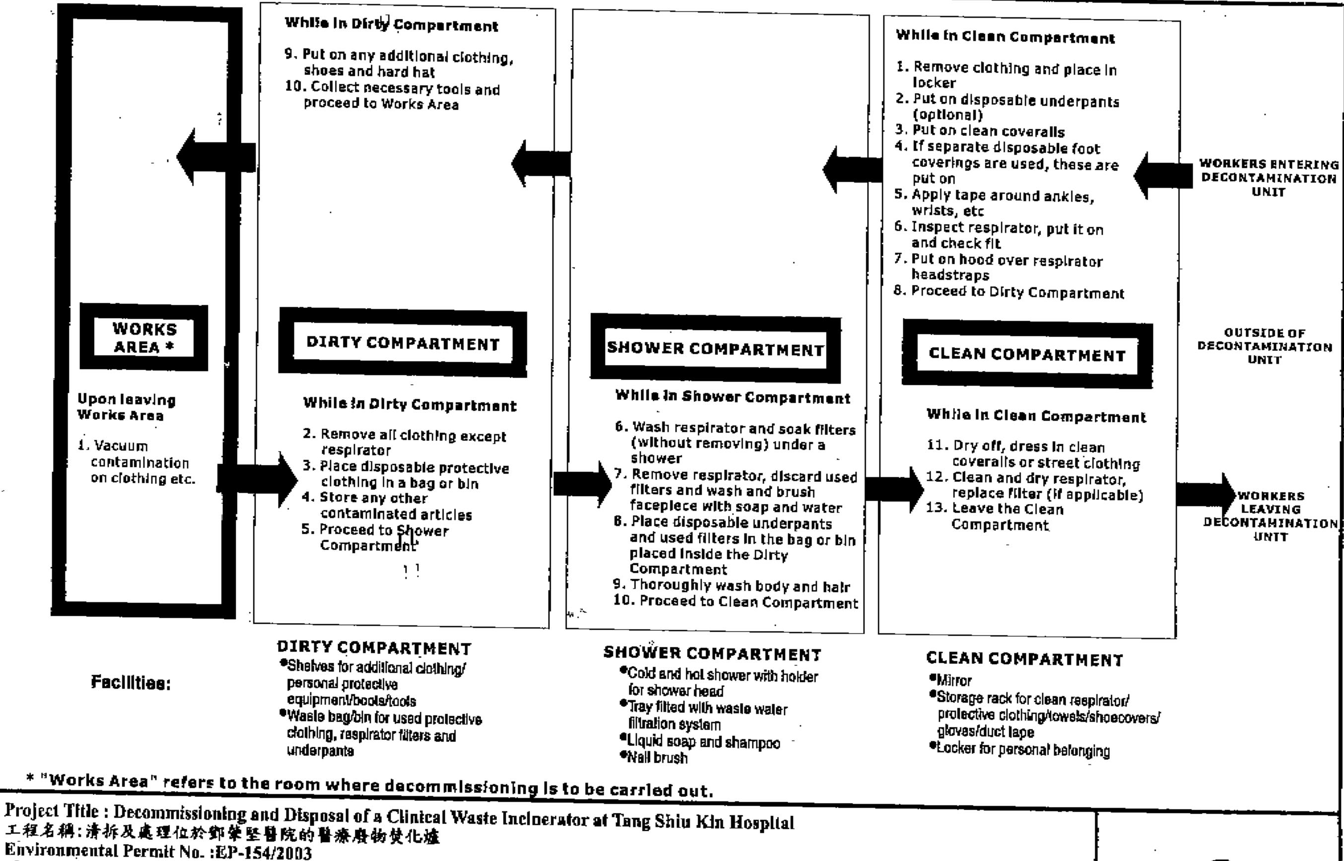
環境許可證論號:EP-154/2003 Figure 5: Procedures for Entering and Leaving 3-Chamber Decontamination Unit
