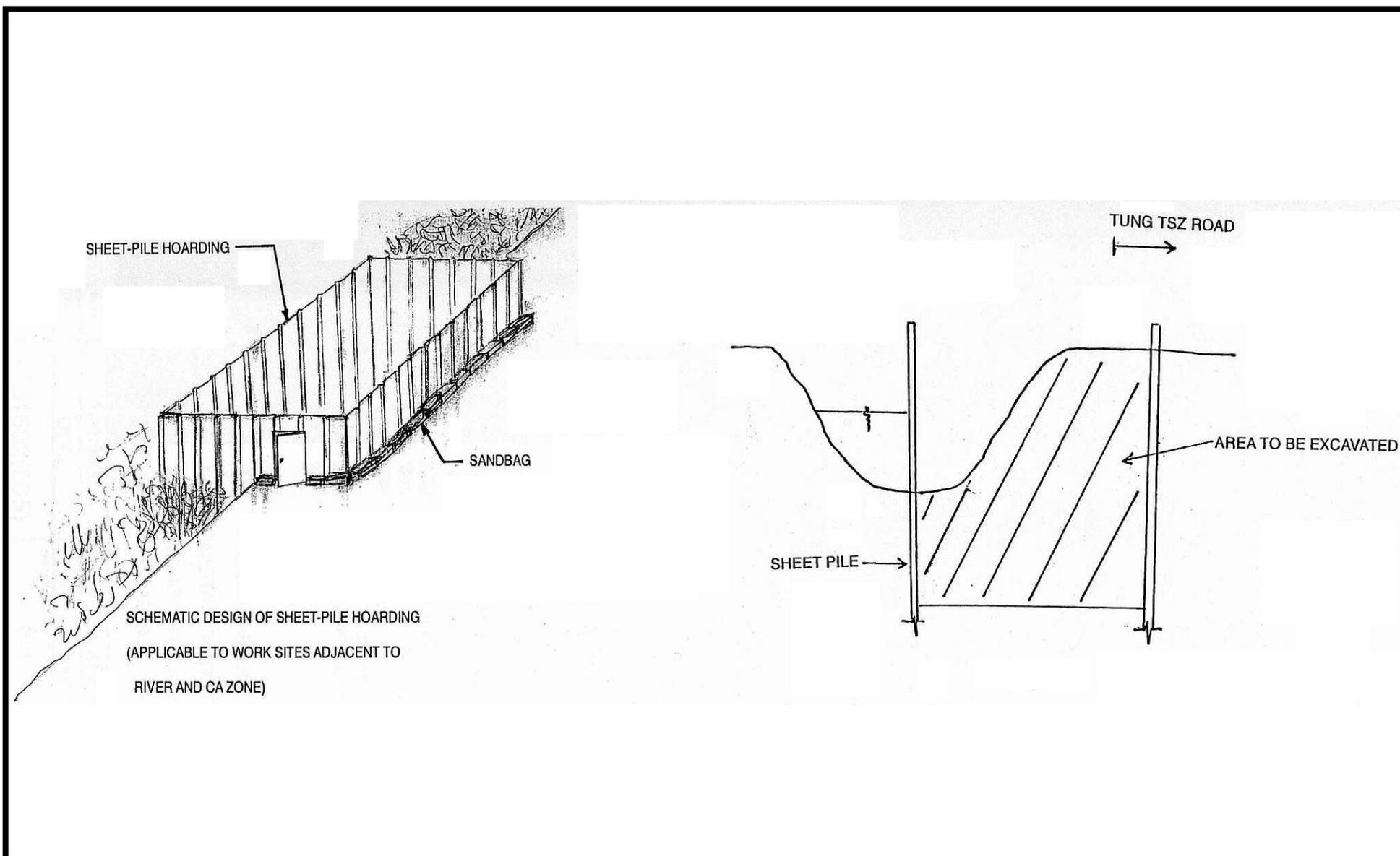
Figure 2 Schematic diagram showing the arrangement of hoardings and sanbags during construction of the box culvert along Tung Tze Road
