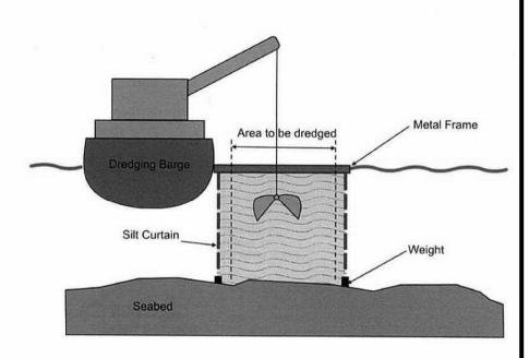
(a) Cage Type Silt Curtain Arrangement for Grab Dredging
