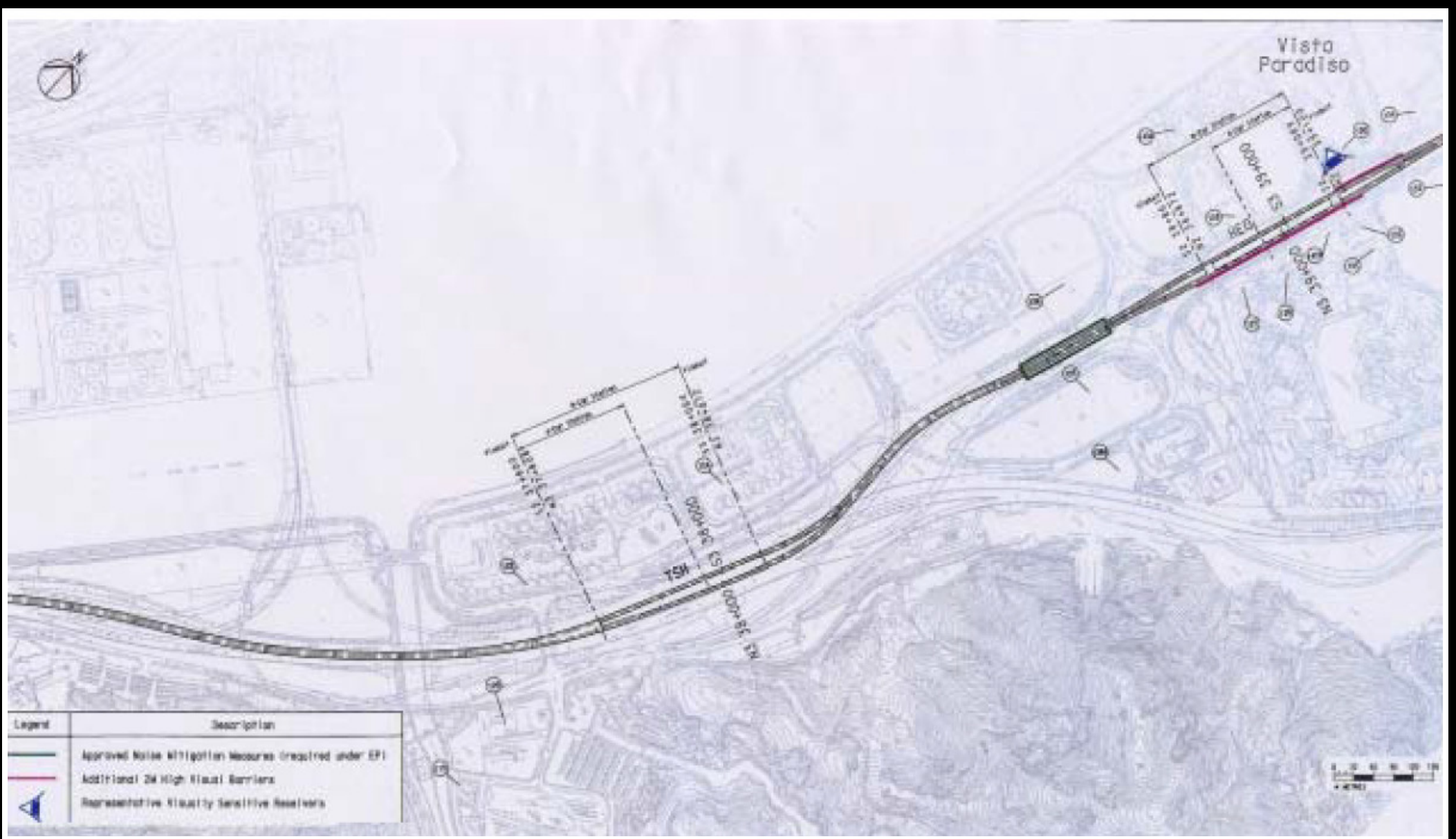
Project Title: East Rail Extensions - Tai Wai to Ma On Shan Figure 28: Locations of Additional 2m High Visual Barriers [Extracted from the Figure 28 of FEP Application (Application No.: FEP-132/2012)]
