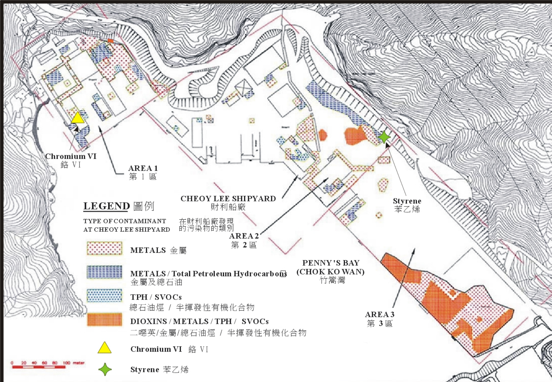
Figure 4 Location of Contaminated Soil
