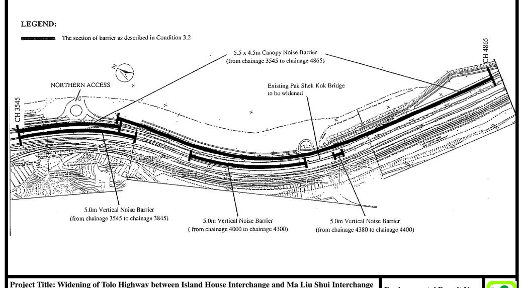
Figure B: Location of Additional Noise Barrier for Pak Shek Kok Development (Extracted from Figure 5, 6 and 7 of the Environmental Permit Application No. VEP-032/2000)
