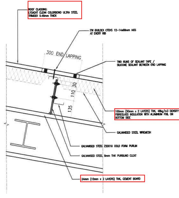
TYPICAL SECTION OF TRIMDEK INSULATED ROOF CLADDING SYSTEM
