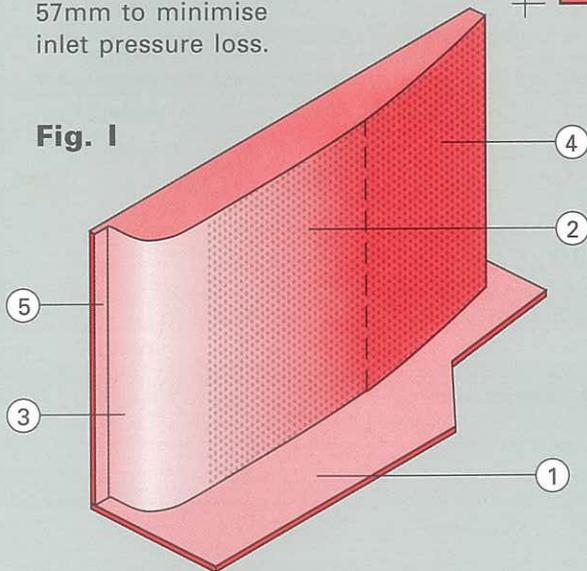
4. 'Evase' shape at baffles' trailing end to achieve static re-gain and optimum attenuation to pressure drop ratio.
