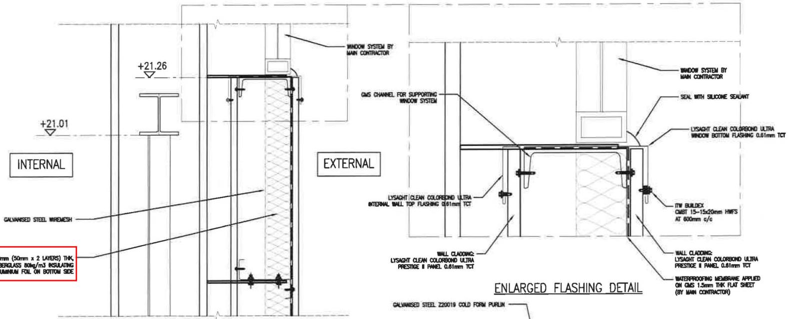
ENLARGED FLASHING DETAIL
