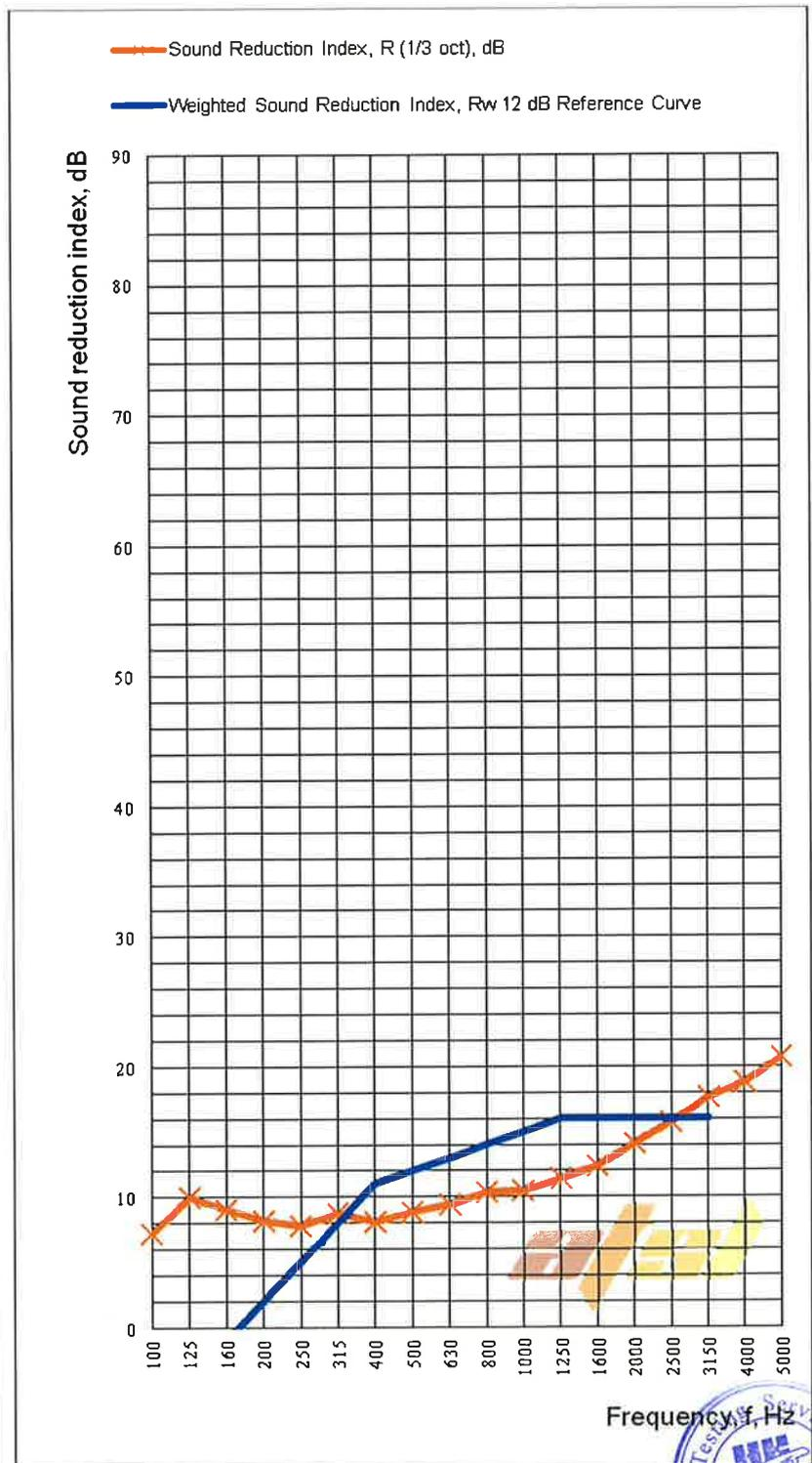
Figure 1. Sound Reduction Indexes against Frequency
