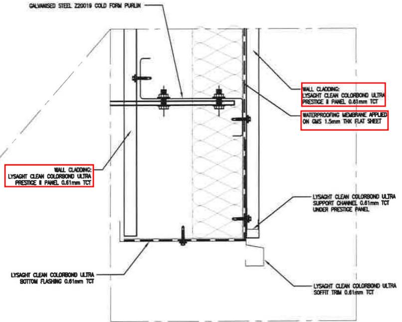
ENLARGED FLASHING DETAIL
