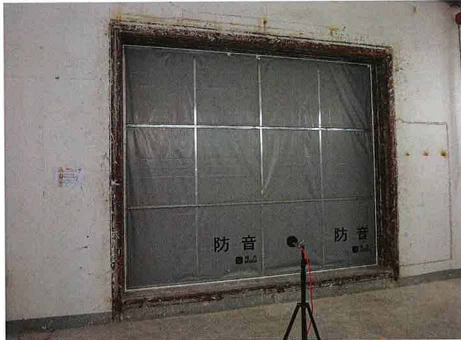
Set-up of Unit Under Test (Source room)
