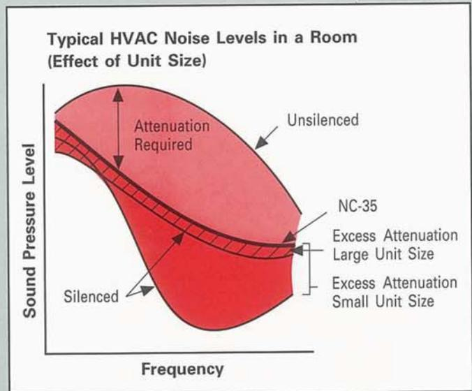
1. Vibron developed the large unit size RDL series of silencers which gives adequate insertion loss at the lower octave bands. This will eliminate over-attenuation at higher octaves while at the same time significantly lower the pressure drop across the silencer, saving energy consumption of the air handler and reduce regenerated noise.
