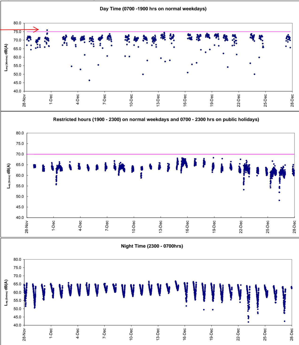
After checking with contractor HY/2009/19, no major noisy construction works were conducted at the concerned location during the recorded period and contractor mitigation measures including erection of temporary noise barrier was confirmed in place. As the exceedance is non-continuous, the exceedances were considered to be contributed by nearby IEC traffic and nearby non- CWB Projects.
