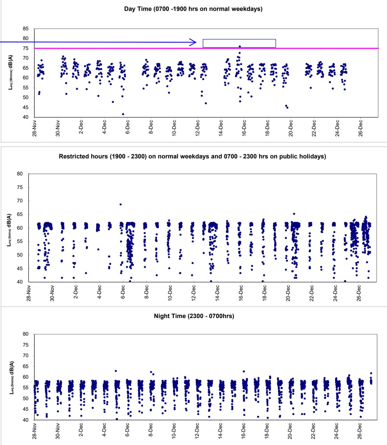
After checking with Contractor of HY/2009/19, on 15 December 2015, concreting was undertaken by Contract HY/2009/19 while steel bar cutting works for Hong Kong Electric Centre was conducted at the roof top by non-CWB Contractor immediately next to the noise monitoring station. In view of the mitigation measures implemented and the non-CWB works conducted next to the monitoring station as major noise contribution, the exceedance was considered as non-Project related.
