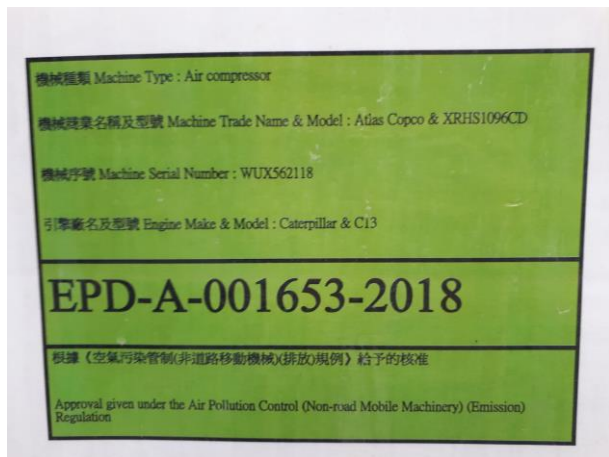
Figure A4 NRMM label on Air Compressor
