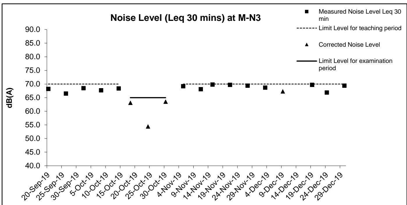
Remark: Corrected Noise Level was applied on 18, 24 and 30 October 2019; Corrected Noise Level = Measured Noise Level - Baseline Noise Level (i.e. 67.7 dB(A))
