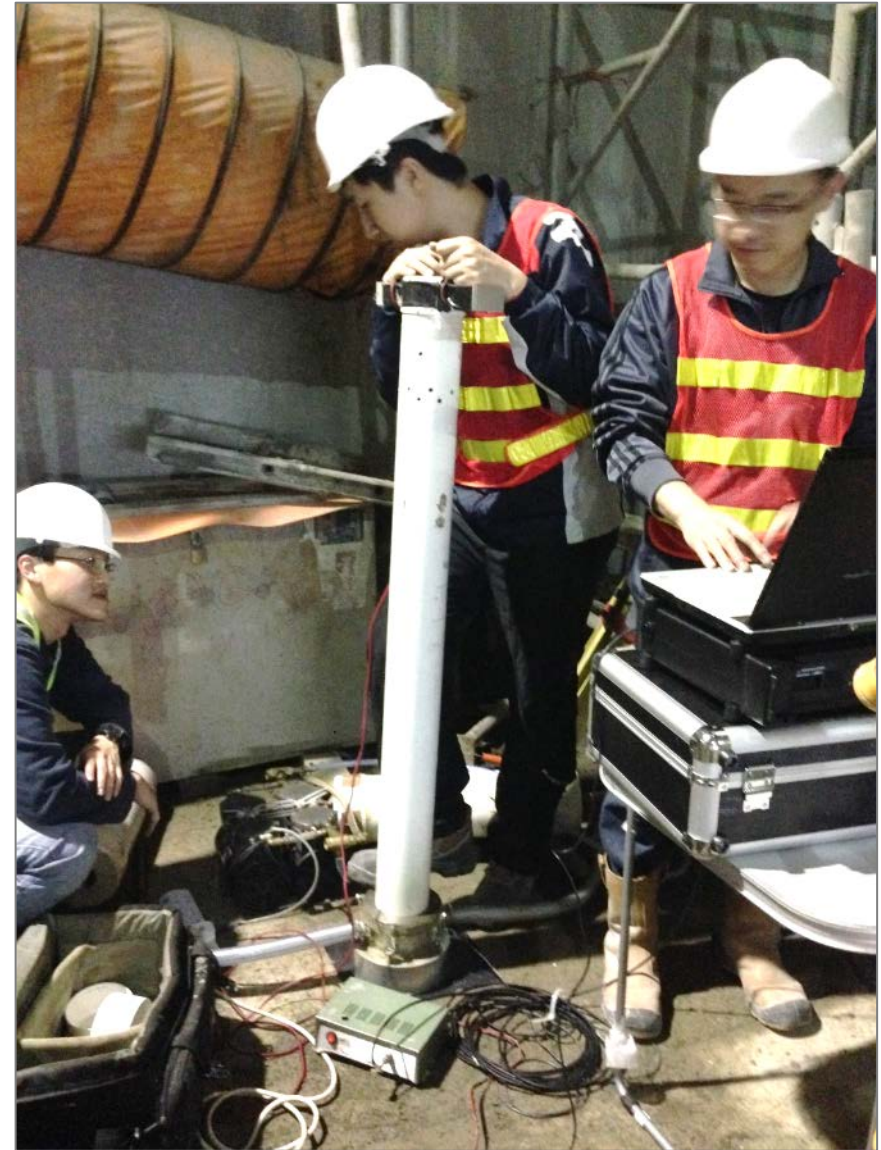
Figure 4.8 Hammer Impact Test at Pt4
