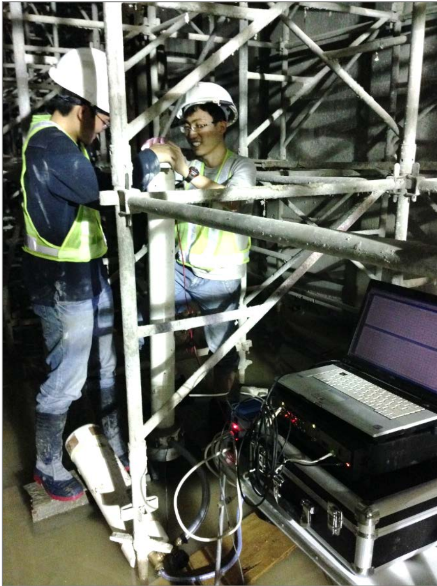
Figure 4.7 Hammer Impact Test at Pt3
