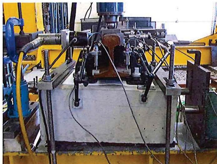
Figure 2.1.2. Vertical static stiffness
