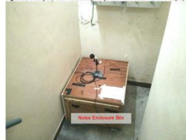
Figure 5.2 Exemplary GBN Monitoring Setup, with Noise Enclosure Box Employed
