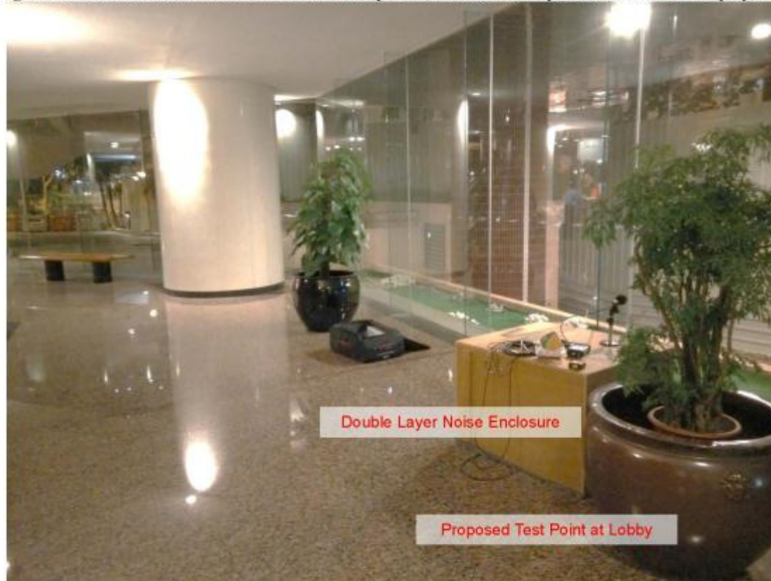
Figure B7. Baseline Measurement at SOH6 on 30-Sep-2015, with Double Layer Noise Enclosure Employed
