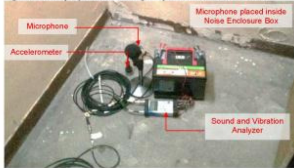
Figure 5.3 Exemplary GBN Monitoring Setup inside Noise Enclosure Box
