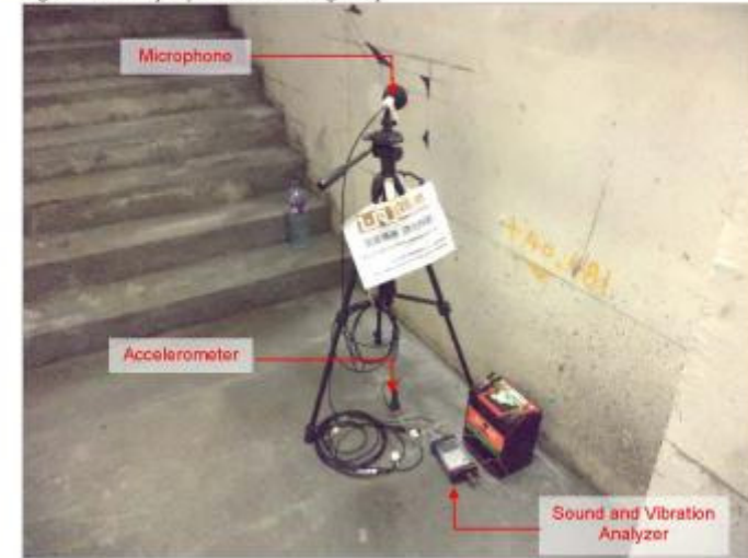
Figure 5.2 Exemplary GBN Monitoring Setup, with Noise Enclosure Box Employed
