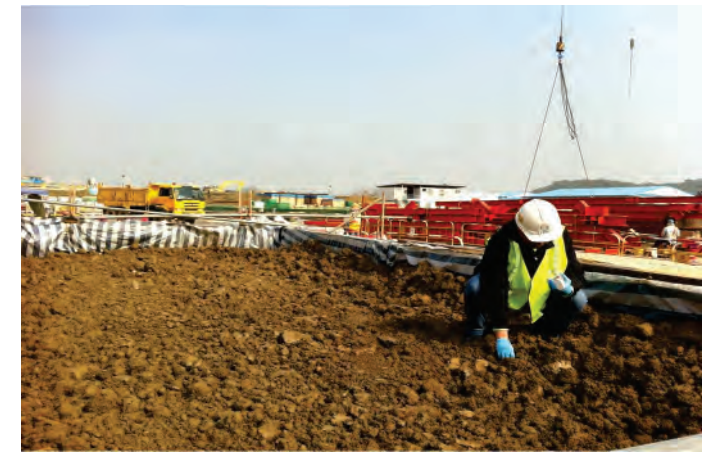
Photo 6: Soil Sampling during monthly remediation progress monitoring.
