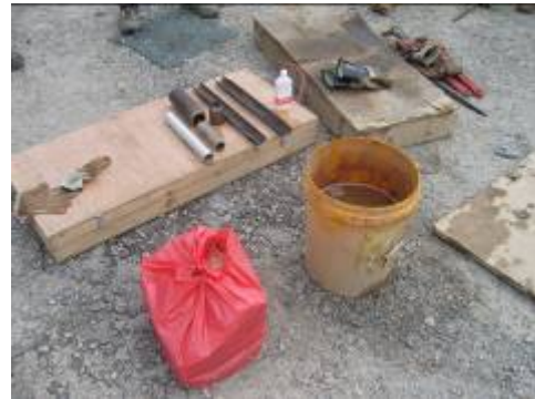
Decontamination of sampling tools.
