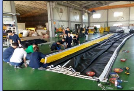
Fabrication of silt curtain
