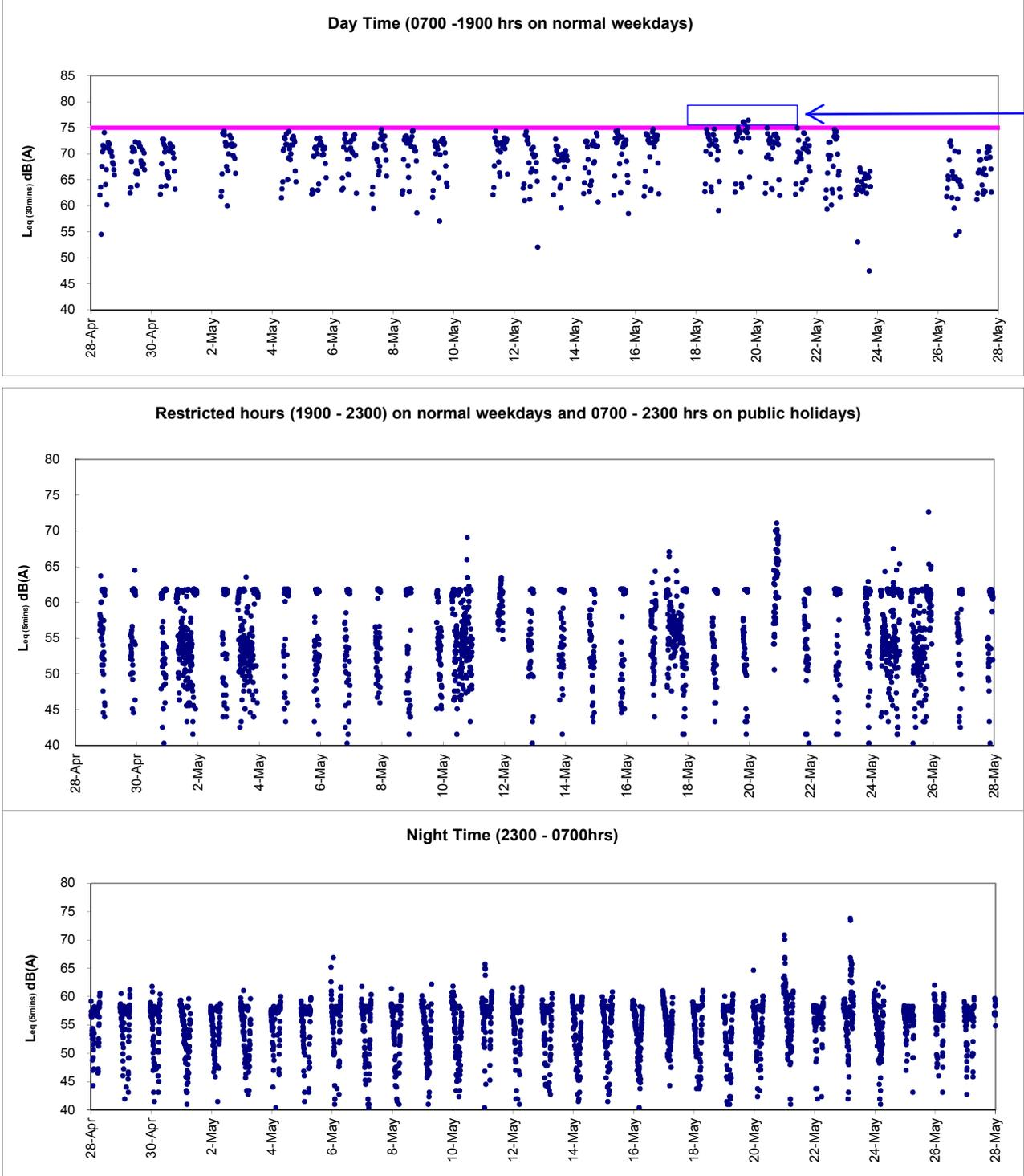
After checking with Contractor of HY/2009/19, U beam lifting works with trailer trucks and crawler crane was conducted on 19 May 2015 and Noise mitigation measures including erection of noise blanket was implemented by the Contractor while breaking works and excavation works was noted on-going at the construction site located next to the monitoring station. In view of the above, the exceedances were considered to be non-Project related and contributed by nearby non-CWB construction site works.
