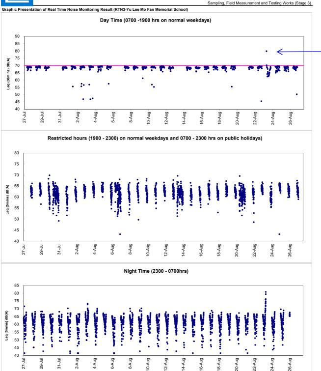
After checking with Contractor of HY/2009/19, no construction works was conducted during the monitoring period with respect to the hoisting of the Typhoon Signal No.8 and the exceedance is considered to be contributed by adverse weather condition. Hence, the exceedance was considered as non-Project related.
