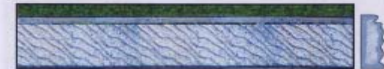
Channel lining with texture treatment to concrete surface
