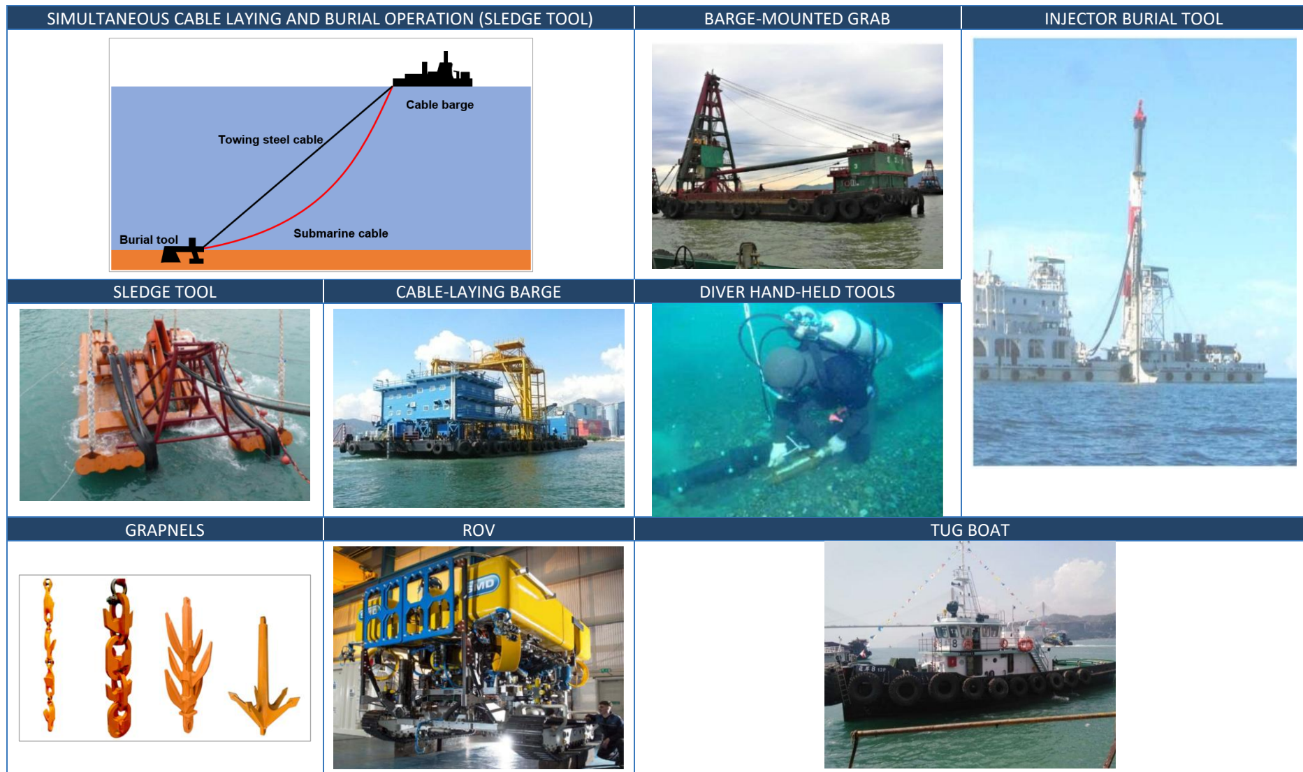
Figure 2-4 Examples of Cable-laying Barge and Cable Burial Tools
