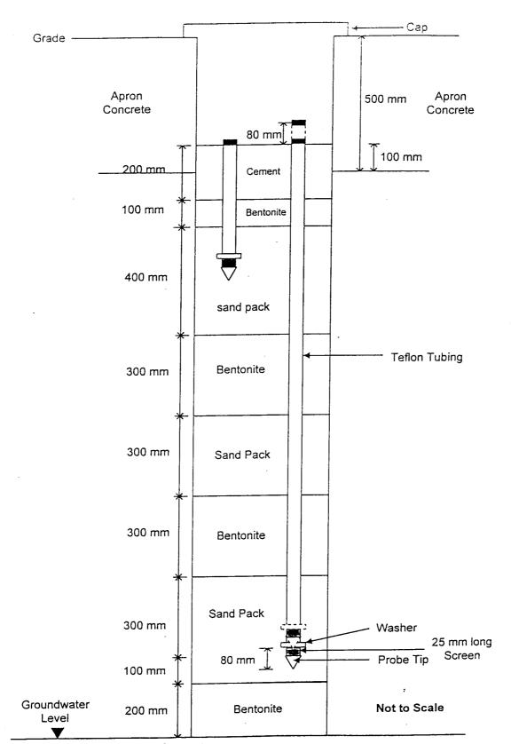
Note: All deep probes and deep probes A2 & E2 had been pulled up for 80 mm before commencement of Long-term SVE tests (re-test) at VT2 and VT3 respectively. The surface seals were then repaired immediately.
