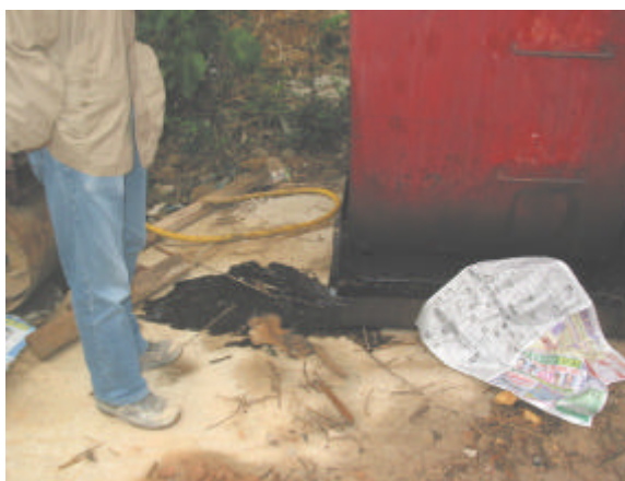
Figure 6-2 - Oil leakage at Gate 10 Storage Yard
