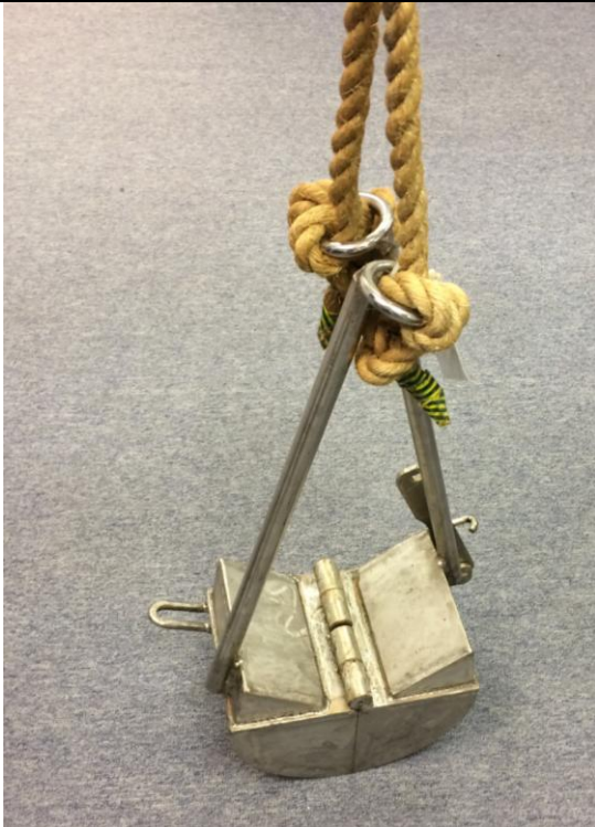
Photo 1. A polar grab sampler
