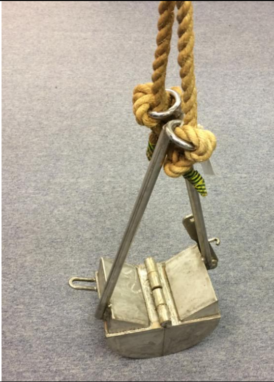
Photo 1. A ponar grab sampler
