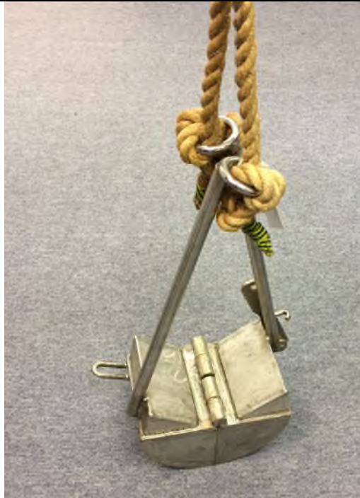
Photo 1. A polar grab sampler
