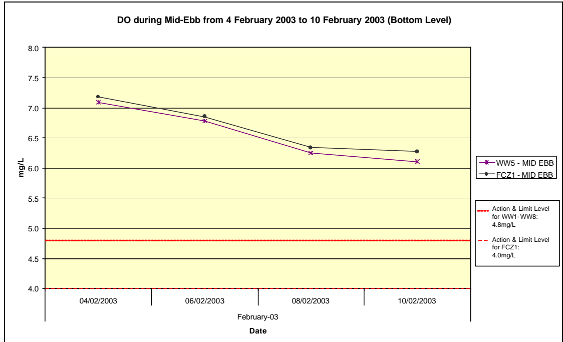
Figure 6-7 DO at bottom level during mid-ebb from 4 February 2003 to 10 February 2003
