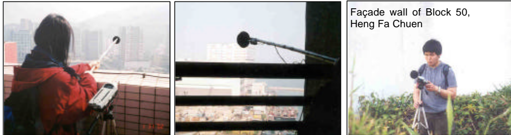
Figure 3-1 Noise monitoring in progress
