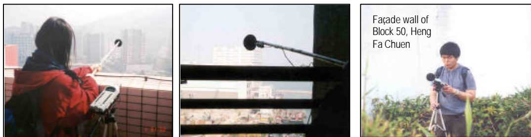
Figure 3-1 Noise monitoring in progress
