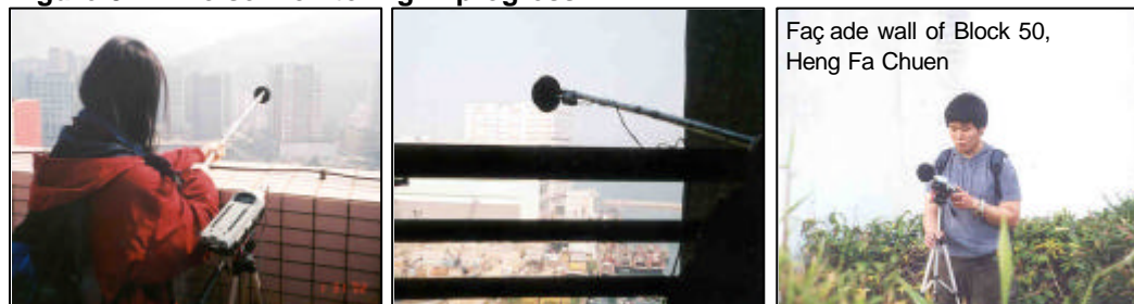
Figure 3-1 Noise monitoring in progress
