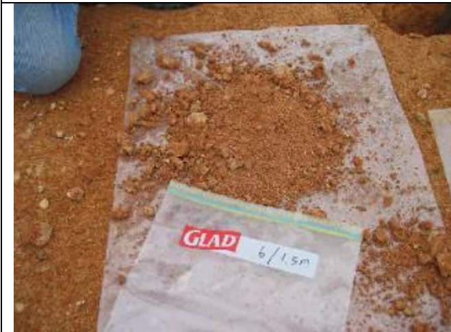
Soil sample taken at depth of 1.5m at location L6
