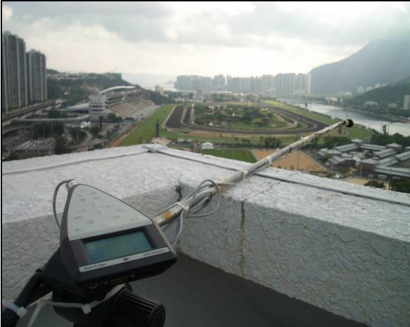
Photo 1: Sound level meter and microphone set-up at Chun Cheung Court, HKJC Staff Quarter (NM1).
