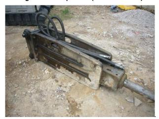
Oil leakage was observed from the breaker, the contractor was requested to provide mitigation to prevent contamination.
